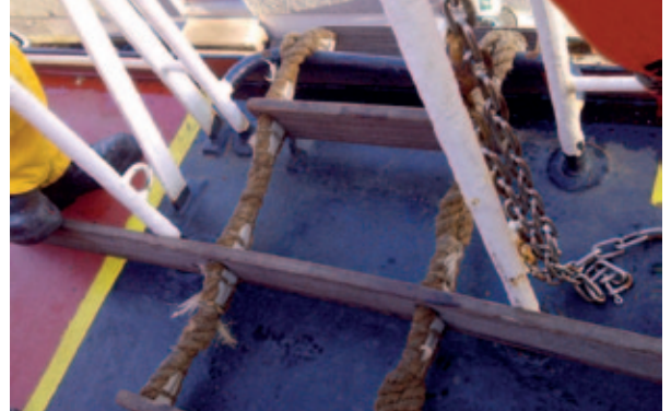
Poor and incorrect securing method
